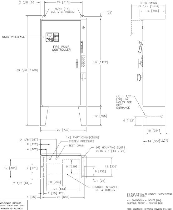
STANDARD WITHSTAND RATINGS 200-600V - 100,000 Amps RMS Sym INTERMEDIATE WITHSTAND RATINGS 200-600V - 150,000 Amps RMS Sym. HIGH WITHSTAND RATINGS 200-600V - 200,000 Amps RMS Sym
