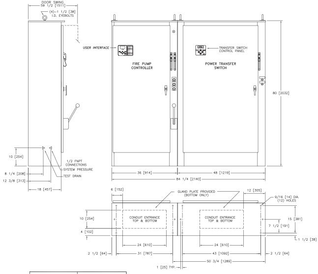
STANDARD WITHSTAND RATINGS 200-600V 100,000 Amps RMS Sym. INTERMEDIATE WITHSTAND RATINGS 200-600V 150,000 Amps RMS Sym. HIGH
