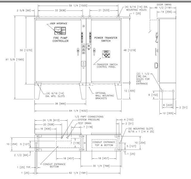
STANDARD WITHSTAND RATINGS 200-600V - 100,000 Amps RMS Sy 200-600V - 100,000 Amps RMS Sym.
