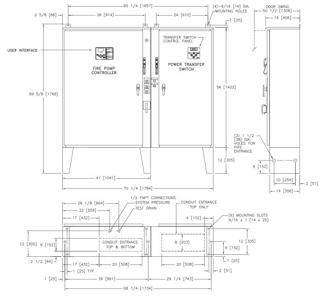
STANDARD WITHSTAND RATINGS 200-600V - 100,000 Amps RMS Sym INTERMEDIATE WITHSTAND RATINGS
