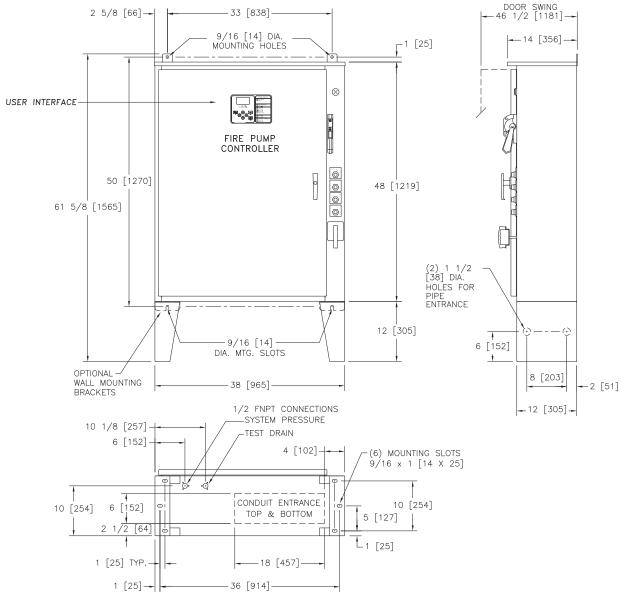
STANDARD WITHSTAND RATINGS 200-600V - 100,000 Amps RMS Sym. INTERMEDIATE WITHSTAND RATINGS 200-600V - 150,000 Amps RMS Sym. HIGH WITHSTAND RATINGS
