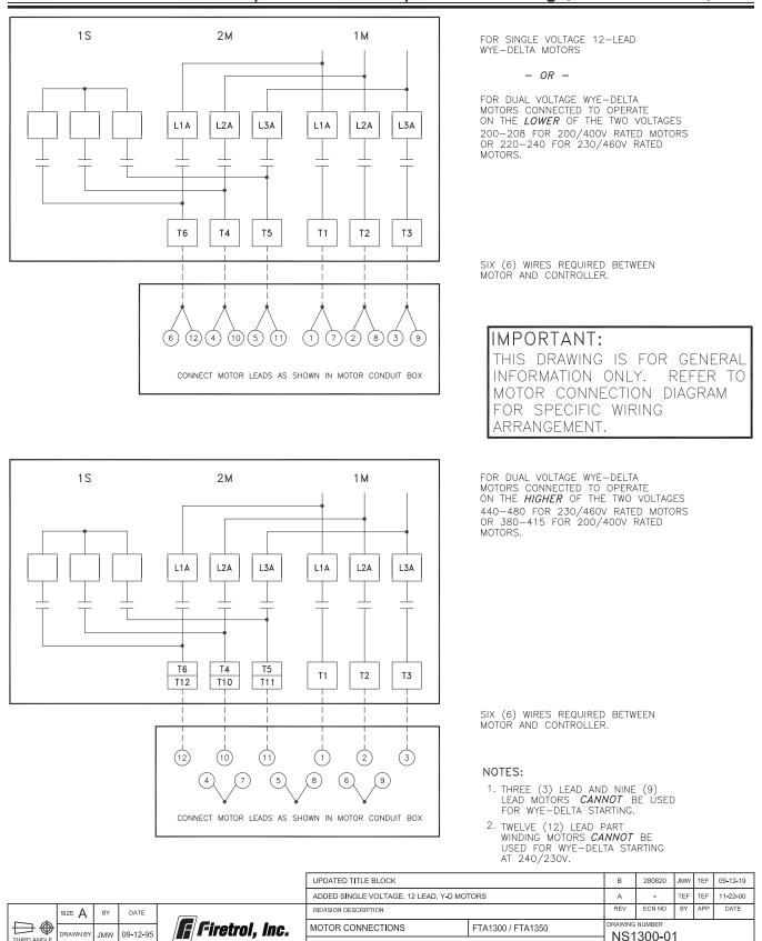
OPEN/CLOSED TRANSITION WYE-DELTA FIRE PUMP CONTROLLERS
