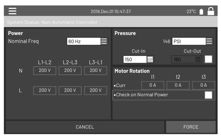
Once the controller has booted up, the "First Start Up" page appears. The controller will automatically detect and display the frequency of the power source. It is then possible to manually choose the frequency of the voltage.
