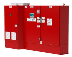
**Description** – Firetrol® Variable Speed Electric Fire Pump Controllers provide a variable frequency drive (VFD) in a PID process control loop to control the speed of a centrifugal pump for the purpose of limiting system pressure in a fire sprinkler system. These controllers are available in the following configurations:
