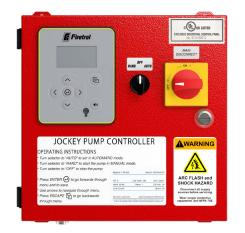
**Description**—Firetrol® FTA570F Jockey Pump Controllers are intended for use with fire pump systems. They are used for pressure maintenance in fire pump installations to prevent unnecessary operation of the main fire pump.
