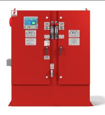
**Description**—Firetrol® FTA750 Limited Service Controllers are intended for use with small electric motor driven fire pumps where the capacity of the power source permits full voltage starting. Full voltage is applied to the motor as soon as the controller is actuated. The controller monitors, displays and records fire pump system information.
