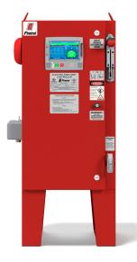
**Description**—Firetrol® FTA750 Limited Service Controllers are intended for use with small electric motor driven fire pumps where the capacity of the power source permits full voltage starting. Full voltage is applied to the motor as soon as the controller is actuated. The controller monitors, displays and records fire pump system information.
