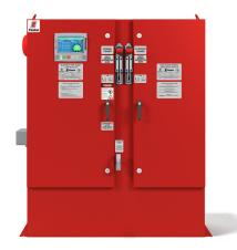
**Description**—Firetrol® FTA750 Limited Service Controllers are intended for use with small electric motor driven fire pumps where the capacity of the power source permits full voltage starting. Full voltage is applied to the motor as soon as the controller is actuated. The controller monitors, displays and records fire pump system information.
