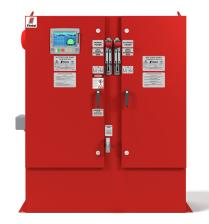
**Description** – Firetrol® FTA1000 Full Voltage Fire Pump Controllers are intended for use with electric motor driven fire pumps where the capacity of the power source permits full voltage starting. Full voltage is applied to the motor as soon as the controller is actuated. The controller monitors, displays and records fire pump system information.
