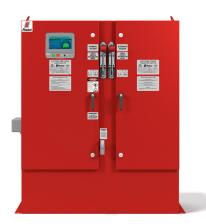
**Description**—Firetrol® FTA1250 Part Winding Starting Fire Pump Controllers can be used where the characteristics of the power source do not permit full voltage starting. The controller monitors, displays and records fire pump system information.
