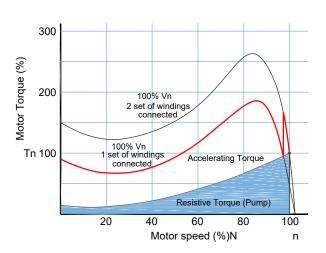
**Starting Method:** Part Winding **Starting voltage per winding:** Full
