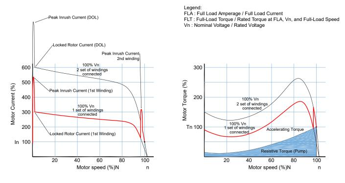
Starting Method: Part Winding Starting voltage per winding: Full Typical voltage applied at motor starting (%Vn): 100% Peak inrush current at starting <sup>(1)</sup>: 5 - 14 x FLA Peak inrush current at transition <sup>(1)</sup>: (2 - 5) x FLA Starting current (% FLA) <sup>(2)</sup>: 250 - 500% Transition current (% FLA) <sup>(3)</sup>: 250 - 500% Starting Torque (% FLT) <sup>(4)</sup>: 25 - 75% Motor type: 6 winding Number of wire connections: 6
