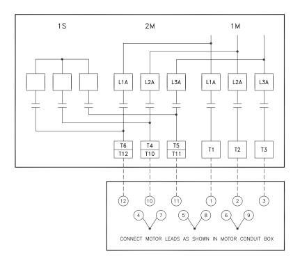
FOR DUAL VOLTAGE WYE-DELTA MOTORS CONNECTED TO OPERATE ON THE *HIGHER* OF THE TWO VOLTAGES 440-480 FOR 230/460V RATED MOTORS OR 380-415 FOR 200/400V RATED MOTORS.
