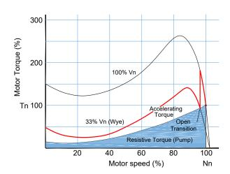
**Starting Method:** Wye-Delta open transition **Starting voltage per winding:** Reduced
