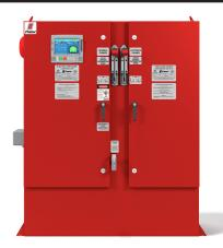
Description—Firetrol® FTA1300 Wye-Delta, Open Transition Starting Fire Pump Controllers are used with delta-wound squirrel cage motors. FTA1300 controllers are of the open circuit transition type in which the motor circuit is opened during the transition from start to run. The controller monitors, displays and records fire pump system information.
