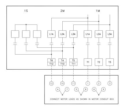
FOR DUAL VOLTAGE WYE-DELTA MOTORS CONNECTED TO OPERATE ON THE *HIGHER* OF THE TWO VOLTAGES 440-480 FOR 230/460V RATED MOTORS OR 380-415 FOR 200/400V RATED MOTORS.
