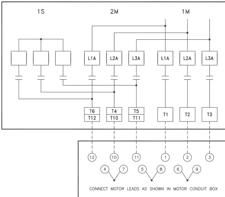
FOR DUAL VOLTAGE WYE-DELTA MOTORS CONNECTED TO OPERATE ON THE **HIGHER** OF THE TWO VOLTAGES
