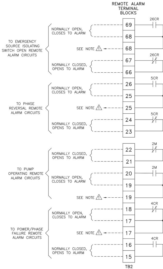
△ SPARE TERMINALS PROVIDED FOR PARALLEL CONNECTION OF REMOTE ALARMS (IF REQUIRED)
