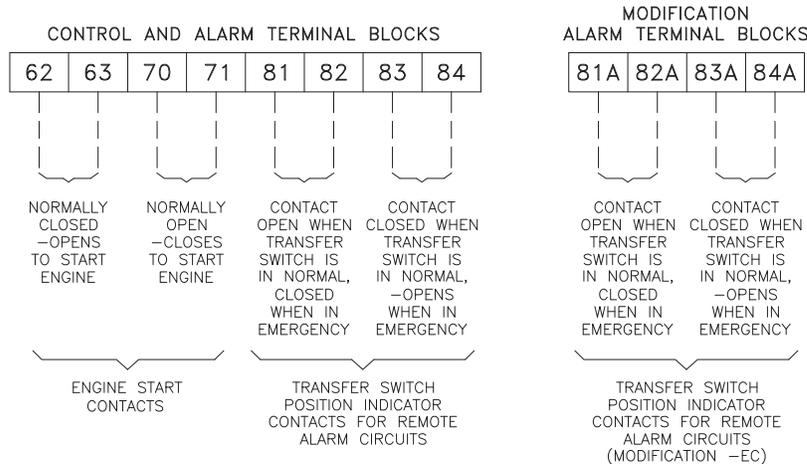
**NOTE:** CONTROL AND ALARM TERMINALS FOR CUSTOMER CONNECTIONS REQUIRE 3.5MM SLOTTED SCREW DRIVER
