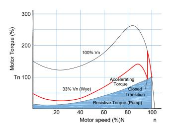
Starting Method: Wye-Delta closed transition Starting voltage per winding: Reduced Typical voltage applied at motor starting (%Vn): 100% Peak inrush current at starting<sup>(1)</sup>: 3.5 - 9 x FLA Peak inrush current at transition<sup>(1)</sup>: Negligible Starting current (% FLA)<sup>(2)</sup>: 165 - 330% Transition current (% FLA)<sup>(3)</sup>: 165 - 330% Starting Torque (% FLT)<sup>(4)</sup>: 20 - 50% Motor type: Standard Wye-Delta Number of wire connections: 6
