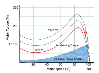
**Starting Method:** Autotransformer **Starting voltage per winding:** Reduced
