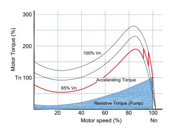
Starting Method: Autotransformer Starting voltage per winding: Reduced Typical voltage applied at motor starting (%Vn): 65% Peak inrush current at starting <sup>(1)</sup>: 4 - 11 x FLA Peak inrush current at transition <sup>(1)</sup>: 4 - 11 x FLA Starting current (% FLA) <sup>(2)</sup>: 210 - 420% Transition current (% FLA) <sup>(3)</sup>: 210 - 420% Starting Torque (% FLT) <sup>(4)</sup>: 40 - 85% Motor type<sup>(5)</sup>: Standard Number of wire connections: 3
