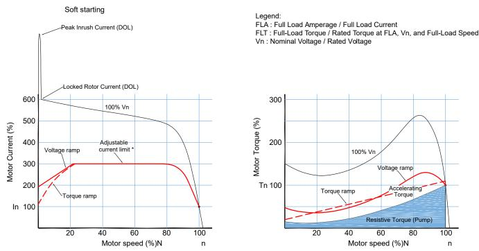
\*Low current limit may cause the motor to not accelerate or even stall; not respecting the 10 seconds ramp code requirement.
