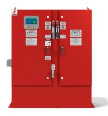
**Description**—Firetrol® FTA1930 Solid State Reduced Current Starting Fire Pump Controllers feature soft start, soft stop and system sensing capabilities that not only provide for reduced current starting, but also offer an improved level of hydro mechanical performance. The controller monitors, displays and records fire pump system information.
