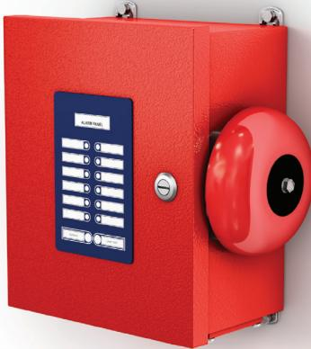
**Description**—Firetrol® FTA200 alarm panels are designed to meet the NFPA 20 specifications requiring a remote alarm panel when the pump house or pump room is not constantly attended. The alarm panel must be installed in a location that is under supervision at all times.
