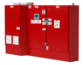
**Description** – Firetrol<sup>®</sup> Variable Speed Electric Fire Pump Controllers provide a variable frequency drive (VFD) to control the speed of a centrifugal pump for the purpose of limiting system pressure in a fire sprinkler system. These controllers are available in the following configurations:
