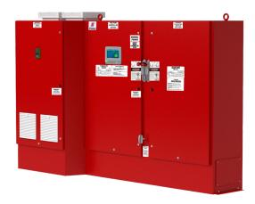
**Description** – Firetrol® Variable Speed Electric Fire Pump Controllers provide a variable frequency drive (VFD) in a PID process control loop to control the speed of a centrifugal pump for the purpose of limiting system pressure in a fire sprinkler system. These controllers are available in the following configurations:
