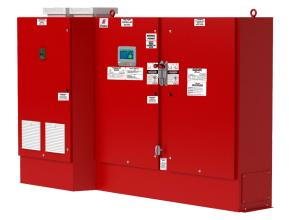
**Description** – Firetrol<sup>®</sup> Variable Speed Electric Fire Pump Controllers provide a variable frequency drive (VFD) in a PID process control loop to control the speed of a centrifugal pump for the purpose of limiting system pressure in a fire sprinkler system. These controllers are available in the following configurations:
