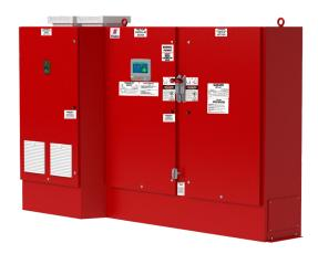
**Description** – Firetrol® Variable Speed Electric Fire Pump Controllers provide a variable frequency drive (VFD) to control the speed of a centrifugal pump for the purpose of limiting system pressure in a fire sprinkler system. These controllers are available in the following configurations:
